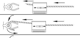
PULL THE RELEASE PIN BACK AND THREAD THE WIRE ROPE INTO ONE LOCK-ING CHANNEL IN THE CABLE LOCK. <u>FAILURE TO PULL ADJUSTMENT PIN FIRST</u> MAY CAUSE DAMAGE TO SERRATED TEETH AND REDUCE HOLDING CAPACITY.
