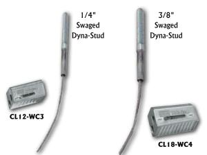
The Dyna-Stud is a heavy duty threaded stud with one end of an aircraft rated cable attached. The stud is threaded into the expansion anchor without putting stress on the cable. This makes for a much safer and tighter connection. The raw end of the cable, in conjunction with the cable lock, is used to attach the object being supported.
