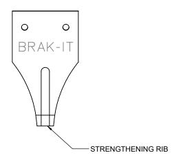
NOTE: The 2.25" may vary due to the material spring back. Not critical to the application of the BRAK-IT)
