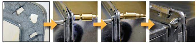
The teardrop shaped cut out of the corner with the proprietary bolt pull the connection together and lock it in place without the use of a nut, using a convenient cordless impact driver.
