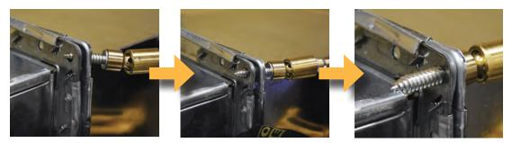
Self-piloting screw tip of the bolt self-aligns the corners and ductwork, eliminating the need for an alignment tool and clamping. 1-1/2" bolt shown.
