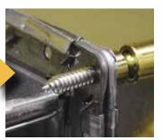
Self-piloting screw tip of the bolt self-aligns the corners and ductwork, eliminating the need for an alignment tool and clamping. 1-1/2" bolt shown.
