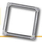
Flange is designed to strengthen the duct wall and connect duct sections together. All Duro Dyne Dyn-O-Mate H Flange is furnished with an <u>integrated sealant pocket</u> for a secure air tight fit and meets SMACNA class H for transverse joints (Aluminum). Bundles of 20ft. lengths are available <u>only</u> with a Full Truckload order and most styles are available in <u>specialty metals</u>. All Dyn-O-Mate Corners that work in the H System are a skid qty of 48 boxes.
