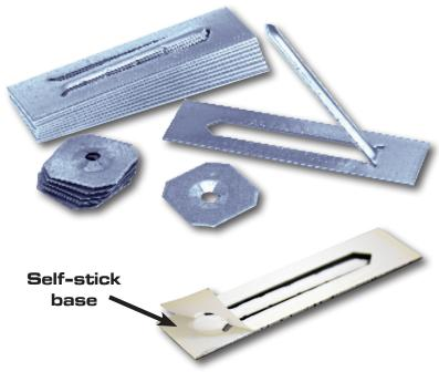
A unique insulation hanger with a self stick base. One fastener can be used for insulation up to 2" thick. Optional extension allows for use on up to 6" thick insulation or wrap. It is the only fastener available in galvanized, aluminum and stainless steel. Insulation can be secured simply by bending the tip of the extended pin or using supplied washers. Flipstix can be used on any clean metal or painted surface and will withstand temperatures of up to 175°F.
