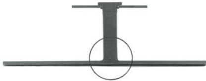
The FG MACH I and MACH IIa utilize Rib Pin™ fasteners which are resistance welded to ductwork securely attaching the fiberglass insulation. Rib Pins are unsurpassed in holding power. In tests conducted by an independent laboratory, samples exhibited holding strength averaging three times that of nail type fasteners.
