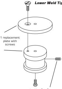
Locking Set Screw (10/32 x 1/4 Socket Head Set Screw)
