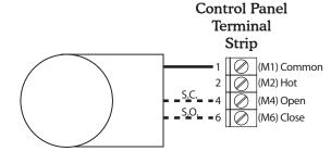
Wiring diagram for a spring return damper.
