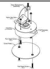
Step 3: Secure the Gear Mechanism Assembly to the Housing using the supplied hardware as shown (Pan-Head Screws and Nylon Hex Nuts). NOTE: The orientation of the Gear Mechanism Assembly may be rotated 90° depending on your available clearance. Secure the Housing in place, then secure the Cover Plate to the Housing using the Flat Head Screws also supplied. (Mounting hardware for the Housing is not Supplied).
