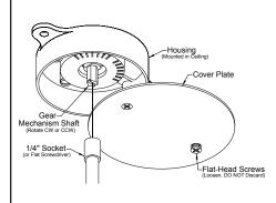
Step 4: Adjusting the Damper Blade "Open" or "Closed" (depending on the starting orientation of the Damper Blade): Using a 1/4" Socket or a Flat Screwdriver, rotate the Gear Mechanism Shaft CW or CCW to the desired position. DO NOT OVER-ROTATE THE GEAR MECHANISM.
