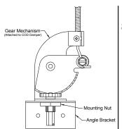
Step 1: Remove but DO NOT discard the Mounting Nut. Remove and discard the Angle Bracket.
