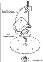
Step 2: Insert the Gear Mechanism into the Rear Mounting Plate as shown. Using a 5/8" Wrench or Deep Socket, secure it with the Mounting Nut from Step-1.
