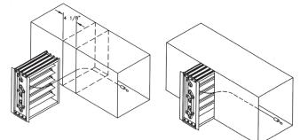
Step 1: Cut 4-1/8" wide slot into the side of the sheet metal duct.
