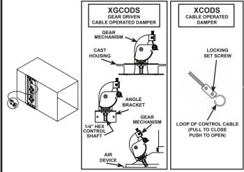
**Step 5:** Route the damper control cable to the remote adjustment point, being sure to avoid severe bending or kinking of the control cable. For XGOCDS, mount gear mechanism to either the wall of the plenum using the angle bracket, or remove the angle bracket and mount it to the air device.
