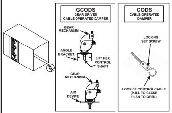
**Step 5:** Pass the damper control cable through the duct to the air device or the remote adjustment point. For GOCDS, mount gear mechanism to either the wall of the plenum using the angle bracket, or remove the angle bracket and mount it to the air device.
