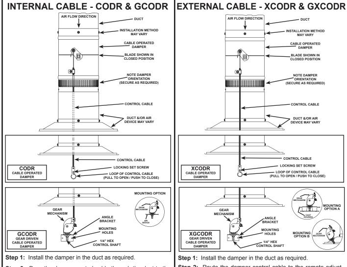
Step 2: Pass the damper control cable through the duct to the air device or the remote adjustment point. For GOCDR, mount gear mechanism to either the wall of the plenum using the angle bracket, or remove the angle bracket and mount it to the air device.
