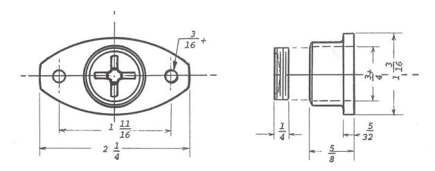
\* NOTE: Whereas the IP-1/1P-2 is "LEAKPROOF" and may be used in High Velocity systems, most test ports are not. In order to render the IP-4 leakproof it is suggested that a dab of pipe-sealing compound be placed on the plug thread after final balancing.
