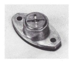
This new, handy Test Port has been designed and produced by Duro Dyne to answer the many requests for a moderately-priced fitting to be used where the superior features of the IP-1 are not required. It offers a 3/4" diameter access to the air stream through a zamac alloy casting set on a neoprene gasket. The screwin cap is readily removed using a standard screwdriver or 25¢ coin.
