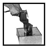
Insert pivot pin. Drill 2nd hole. Begin cut-ting clockwise.
