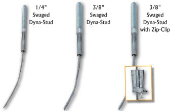
There are many ways to suspend duct work from a concrete or steel structure. One of the most common methods is to screw threaded rod into internally threaded expansion anchors. Sizing the threaded rod and using washers and nuts to complete support structures is time consuming. Dyna-Studs used with Dyna-Tite cable locks can greatly decrease labor time for constructing suspension systems.
