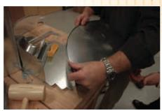
3. Once seam is open insert the second cheek of your ductwork.
