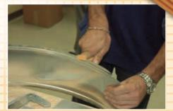
2. Continue this motion along the entire seam until the lock is completely opened.
