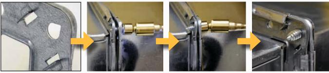
The teardrop shaped cut out of the corner with the proprietary bolt pull the connection together and lock it in place without the use of a nut, using a convenient cordless impact driver. Pictured above is the TDF<sup>®</sup> EZ Corner & 1" bolt.
