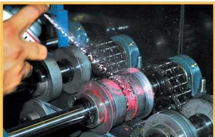
1. Spray The Stripper at those points where galvanizing tends to build up on your machines. The special cleaning ingredients get right to work softening up deposits.
