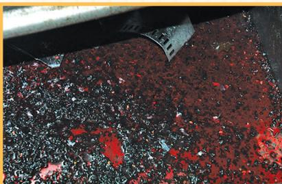
2. Under normal conditions, galvanizing build-up will loosen and flake off by itself after being sprayed with The Stripper. Then if required, remaining build-up can easily be removed by light scraping.
