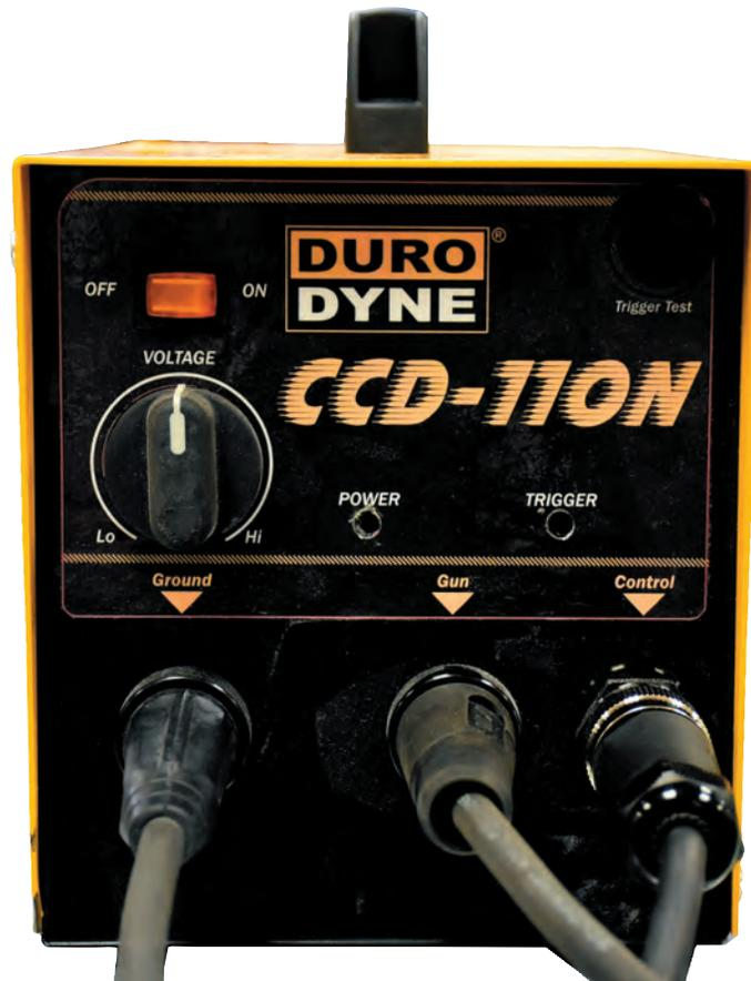
**POWER SWITCH:** The POWER switch applies AC voltage to the power supply Hi/Lo causing the weld capacitors to charge to a voltage level determined by the setting of the VOLTAGE CONTROL. Also, the charge time is dependent on the setting of the VOLTAGE CONTROL, ranging from 1 to 3 seconds.
