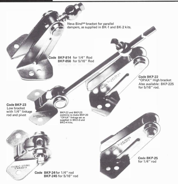
All bracket stampings are of 16 gauge cold-rolled steel, zinc plated. Pivots are made from 1/2" brass rod, set screws are No. 1/4 - 28x1/2" square head, cup point, specially hardened and zinc plated.
